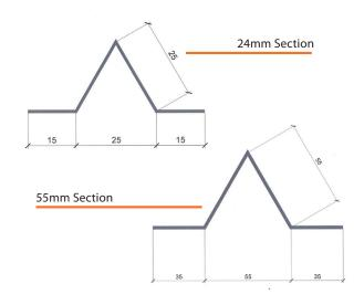
**Notes:** To be used with surface crack control (i.e Crack-A-Joint™, saw-cut). Not to scale.
